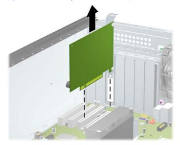
Figure 5-11 Removing a Standard PCI Expansion Card
